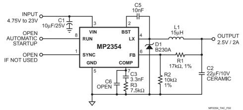
Figure 2—Typical Application Circuit
